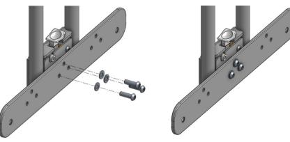
3. Now the rail is ready to be installed onto bed. Insert long countersunk screws through mounting plate and bed spacers
