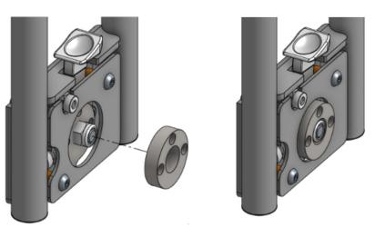
2. Use an Allen key to install the three washers and screws through the circular spacer. Do not overtighten screws
