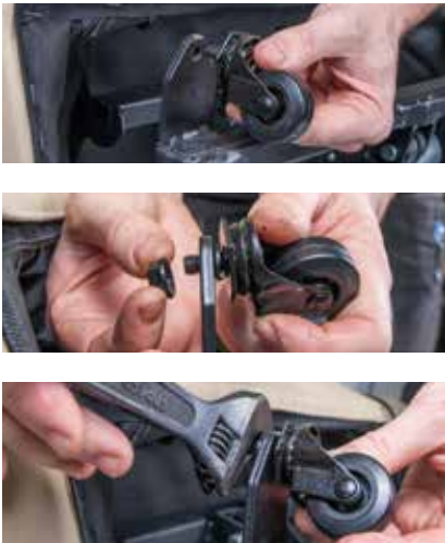
4.3.2 Attach castor stem through plare, lock in place with retaining nut
