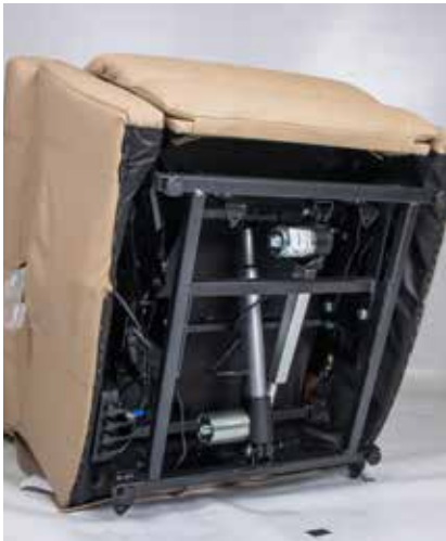
4.3.1 Flip chair onto side to access castor mounts
